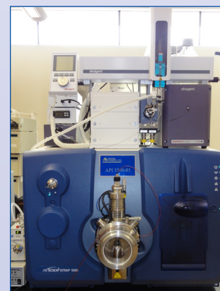
Figure 4. AB SCIEX QTRAP ® 5500 mass spectrometer with Eksigent Express HT-Ultra LC ® MFLC system.
