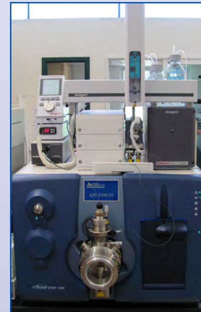
Figure 4. AB SCIEX QTRAP® 5500 Coupled with an Eksigent ekspert™ microLC 200 MFLC System.
