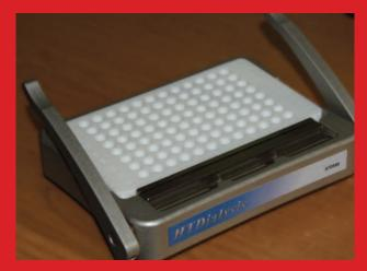
Figure 1: Diagram of a HTDialysis Protein Binding Device
