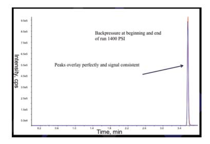
Figure 2. MFLC-MS/MS Chromatograms Overlayed from Beginning and End of Run of >350 injections of MTX Extracted from Human Plasma
