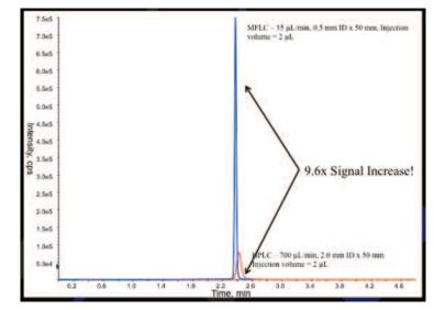
Figure 1. LC-MS/MS Overlayed Chromatograms (HPLC vs. MFLC) from Bioanalysis of Methotrexate (400 ng/mL) from Human Plasma Using Eksigent ekspert microLC 200 and a QTRAP 5500
